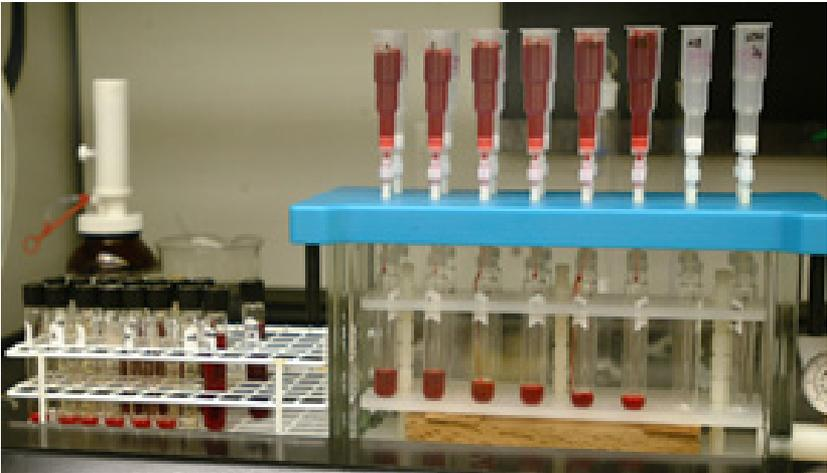
**Fig. 30-1** Manual Solid Phase Extraction and tubes used by the Forensic Toxicologist in preparation for drug confirmation(s).
