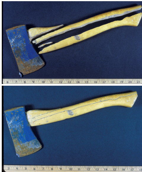
Fig. 24-2 Fracture Match of an axe.
