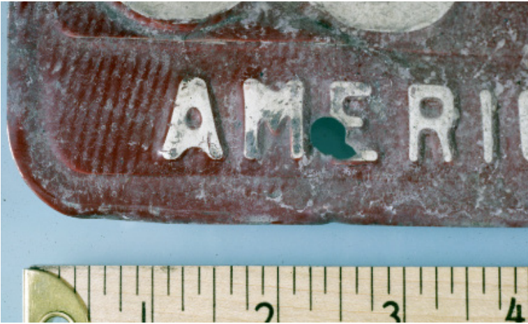
Fig. 22-2 Fabric impression on a license plate from a hit-and-run investigation.
