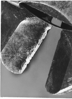
Fig. 19-4: Damage to the cutting edges of the blades creates individual markings on the materials cut by the bolt cutters.
